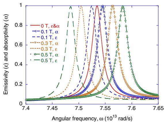
**Fig. 4.** Absorptivity and emissivity spectrum with different magnetic fields at  $\theta = 65^\circ$ . When  $B = 0$  T (the solid red line), the two spectra overlap.
