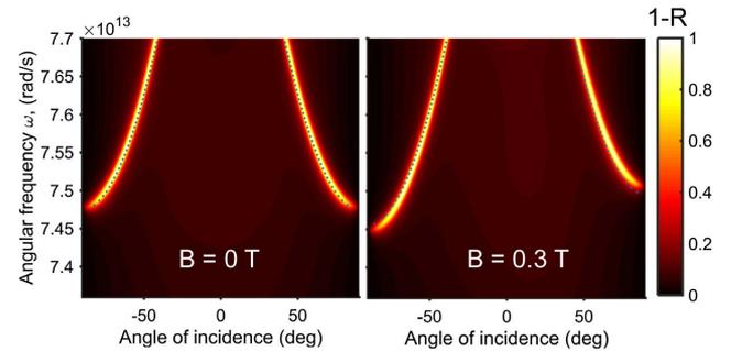
**Fig. 3.** Absorptivity as a function of frequency and angle of incidence for the structure shown in Fig. 1(a) for (a)  $B = 0$  T and (b)  $B = 0.3$  T. The dotted lines are the analytical solution of the dispersion of the guided resonance given by Eq. (6).
