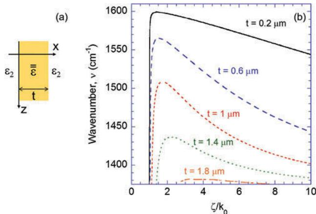
**Figure 5.** (a) Schematic of an anisotropic waveguide made of a uniaxial material with its optical axis in the  $z$ -direction cladded by a dielectric material ( $\epsilon_2$ ). (b) The dispersion curves of the fundamental waveguide mode in a hyperbolic waveguide with different waveguide widths ( $t$ ) when the core material is hBN.
