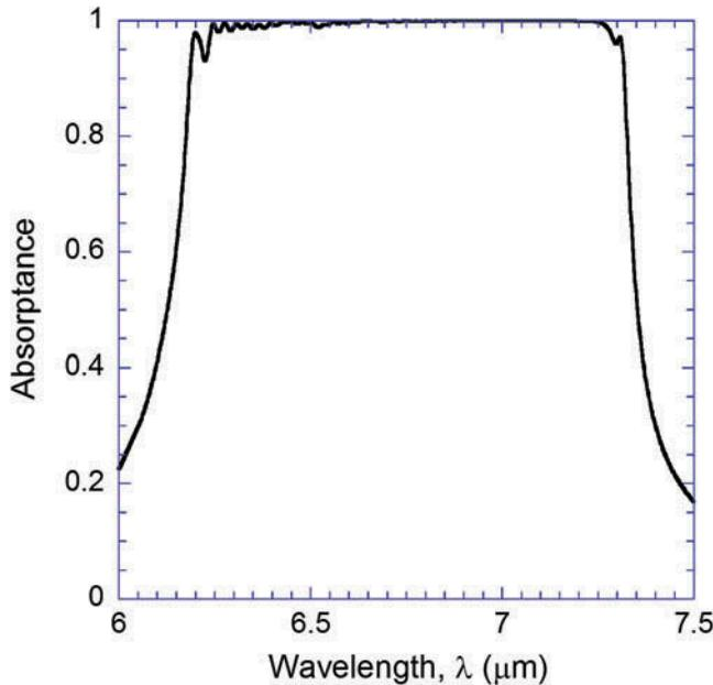
**Figure 2.** Absorptance spectrum for TM waves at normal incidence ( $\theta = 0^\circ$ ) of the proposed structure (shown in the inset) with hBN trapezoidal gratings on an Ag substrate. The grating parameters are  $h = 10 \mu\text{m}$ ,  $\Lambda = 3 \mu\text{m}$ ,  $t_t = 0.04 \mu\text{m}$ , and  $t_b = 2 \mu\text{m}$ .
