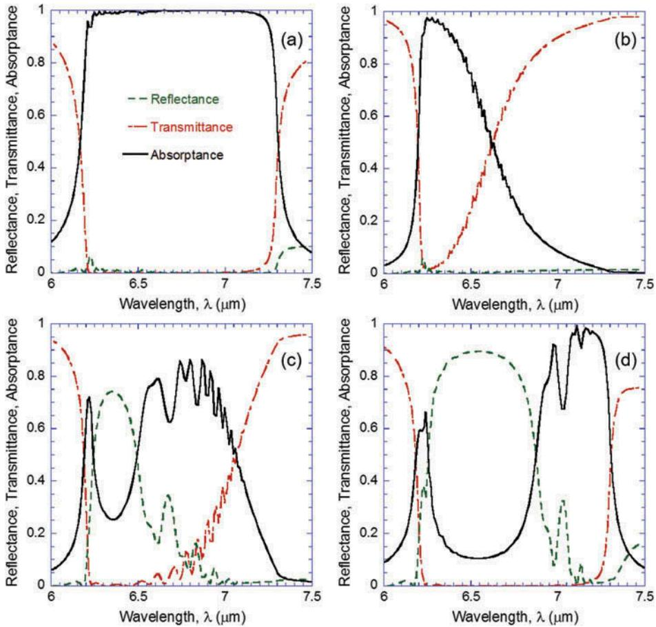
**Figure 7.** Reflectance (dashed line), transmittance (dot-dashed line), and absorptance (solid line) for TM waves at normal incidence ( $\theta = 0^\circ$ ) of four different hBN trapezoid gratings suspended in vacuum: (a) a grating the same geometries as the structure in Figure 2; (b) only the upper half is present; (c) only the middle part is present; and (d) only the lower half is present.
